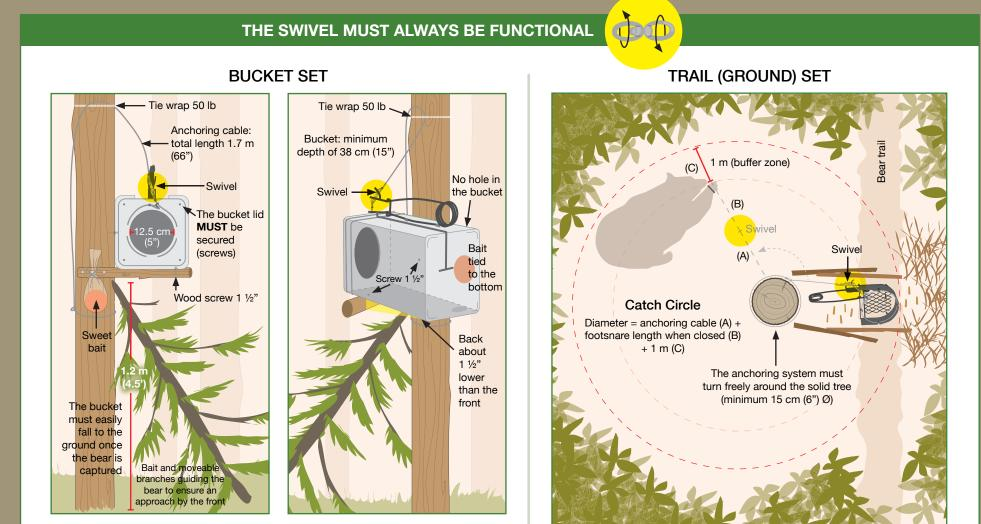
**IMPORTANT:** the anchoring system is the same for both the bucket and the trail set.
